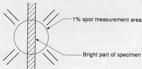
For the specimen as described above, it is necessary to set the 1% measurement mode and make a -1 step or -2 steps exposure compensation. (The degree of correction is based on the ratio of the specimen size to the size of the measurement area. If the ratio is 0.5, the correction value is -1 step.)
