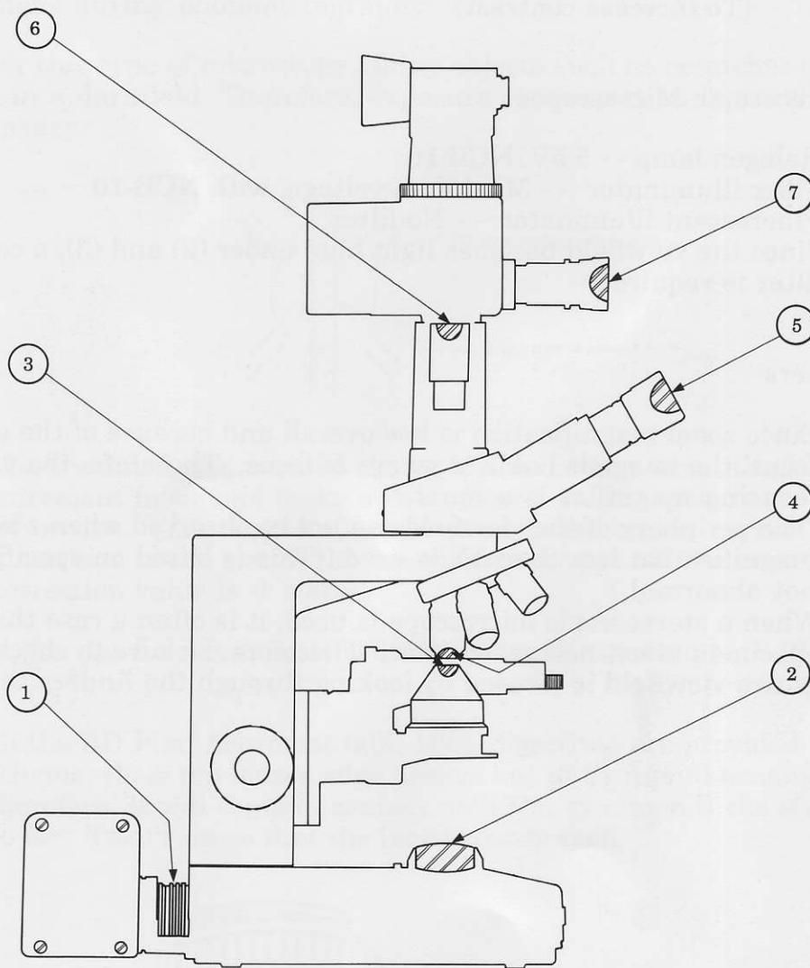
It is recommended that, as a rule, you always clean the seven points indicated above before using a microscope.
