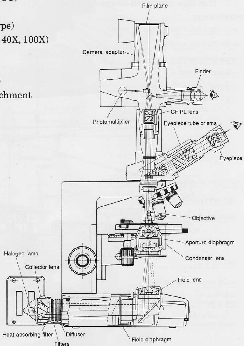
**Optical system in a photomicrographic system**
