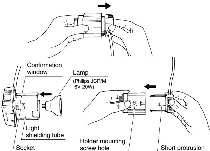
*Note) Do not touch the glass part of a lamp with your bare hands as your skin may burn and stick to the lamp, possibly reducing its level of light output or causing damage to the lamp. When replacing a*
