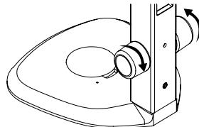
(To reduce the torque, turn the knob in the direction opposite to the arrow.)
