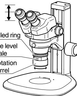
*Note) Changing the eye level will change the magnification. The magnification is 0.77X at the highest eye level, and 1.06X at the lowest eye level. To know the exact magnification, calculate it using the reticle with scaled cross hairs, etc.*
