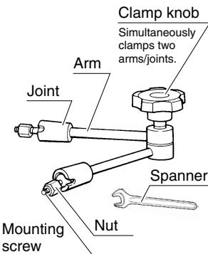
Screw the mounting screw at the other end of the Epi arm into the screw hole on the lamp house in the same manner as described above. Set the lamp house in a position that makes for easy viewing and tighten the clamp knob.
