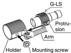
Secure by screwing the mounting screw supplied with the arm into the arm mounting screw hole on the arm of the stand.
