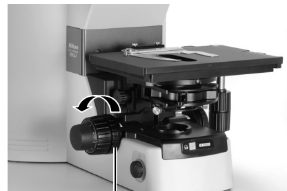
Coarse focus torque adjustment knob
